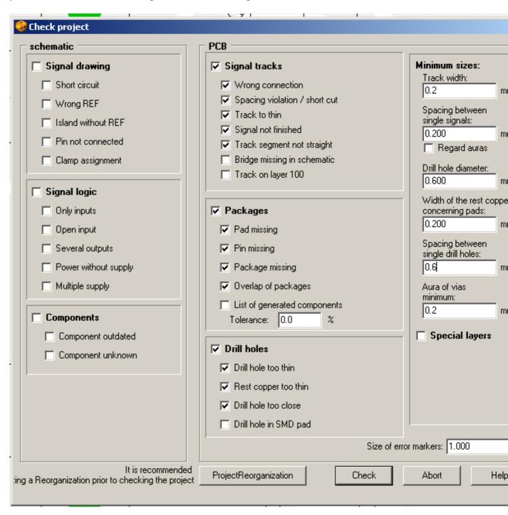
If the DRC check show no errors you can continue with the PCB manufacturig files generation.
